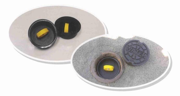
Clogged valve boxes will prevent access to the valve actuating nut and can lead to expensive excavating procedures! Prevent sand, dirt, road salt and other foreign materials from entering your valve box with the Valve Box Insert. Our Valve Box Insert is made of High Density Polyethylene with a minimum thickness of 60 mils. The polypropylene strap is positioned in the center for easy removal and to prevent spillage when removing.
